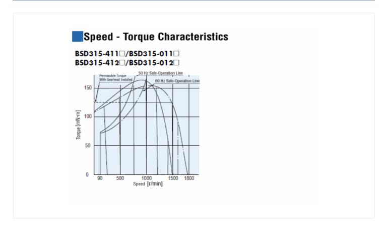
**Speed - Torque Characteristics**
